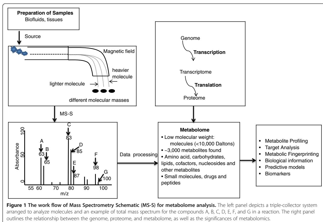
**Figure 1** The work flow of Mass Spectrometry Schematic (MS-S) for metabolome analysis. The left panel depicts a triple-collector system arranged to analyze molecules and an example of total mass spectrum for the compounds A, B, C, D, E, F, and G in a reaction. The right panel outlines the relationship between the genome, proteome, and metabolome, as well as the significances of metabolomics.
